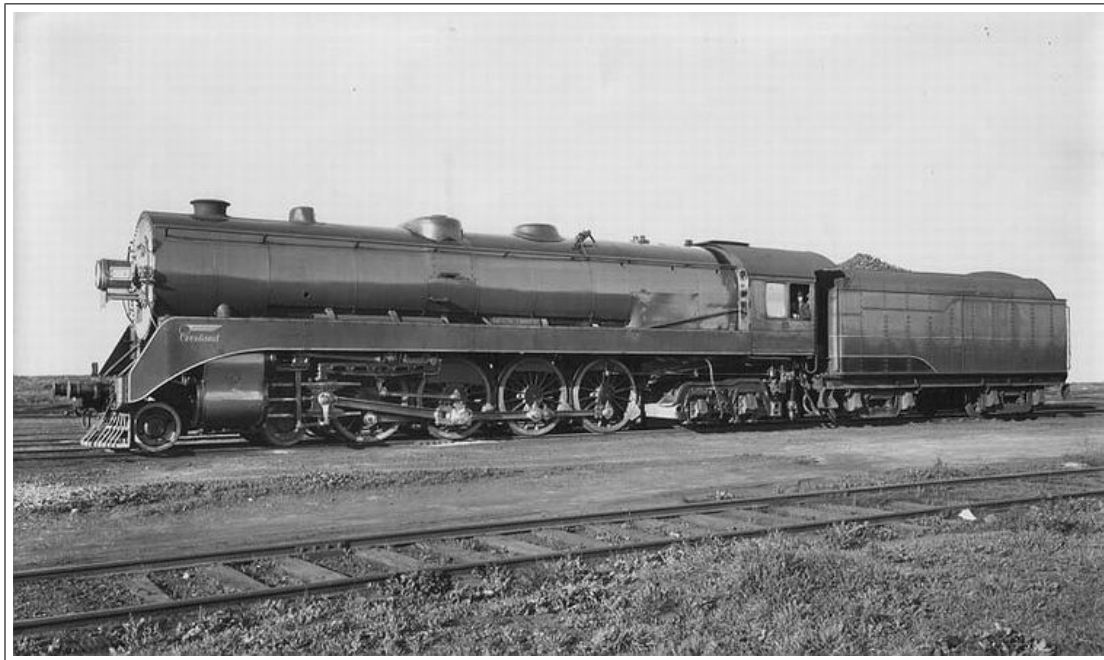
The South Australian Railways 500 class was the biggest of the big power locomotives introduced by Commissioner Webb in the 1920's ( NRM Collection )
