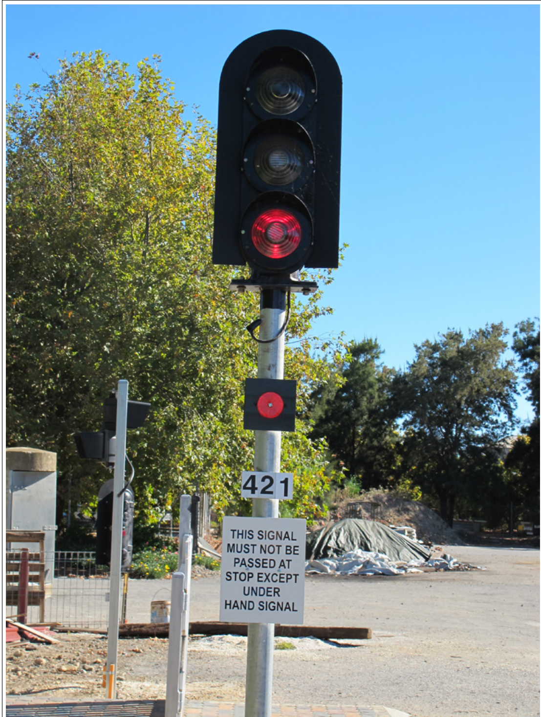
This coloured light signal is used to indicate to a museum train that the warning light on the crossing pedestrian ahead are working - 12 February 2011 ( Chris Drymalik )
