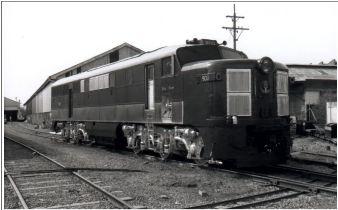
South Australian Railways - 900-class A1A+A1A diesel electric locomotive No. 900 Lady Norrie 20.10.1988 ( R.E.Fluck )
