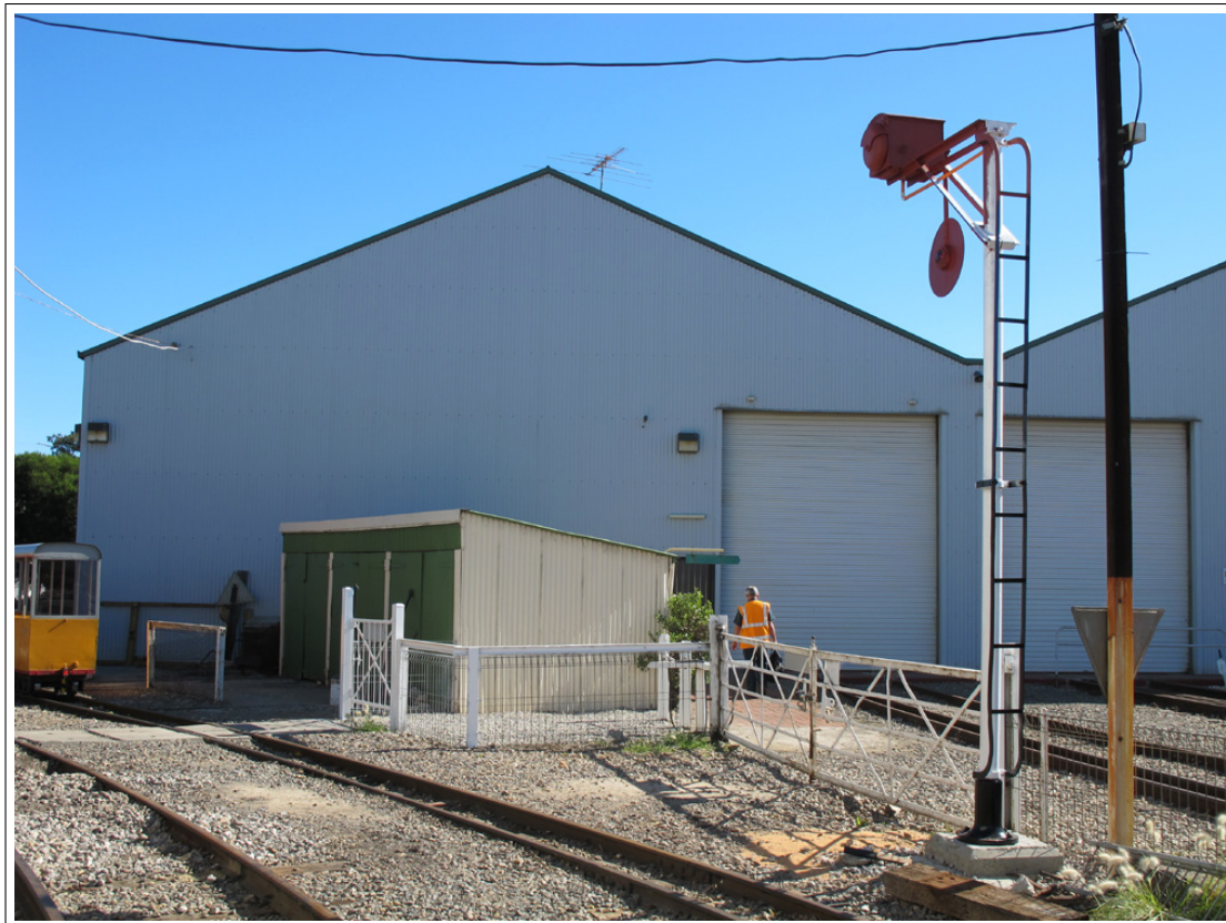
A 'Wig Wag' warning devices protects a crossing gate, adjacent to the Eudunda Quad Shed, at the rear of the Fitch Pavilion - 25th April 2011 ( Chris Drymalik )
