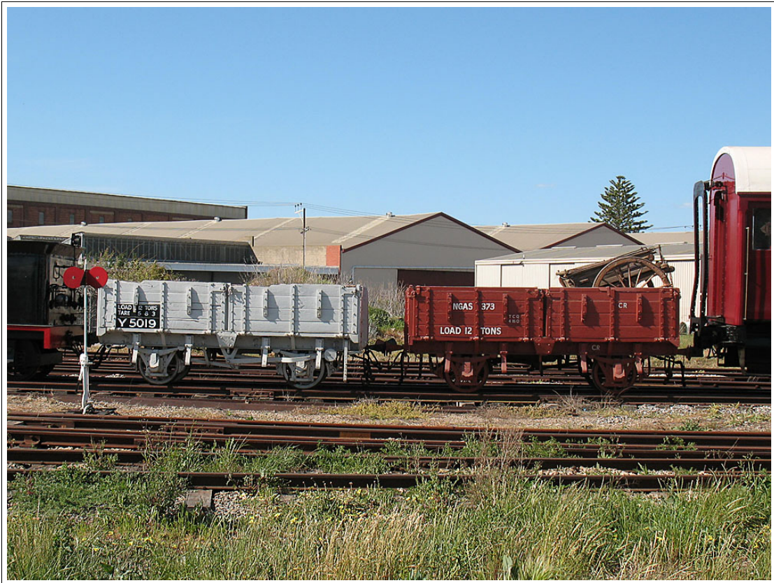
South Australian Railways - Y Class 4-wheel Open wagon (drop-sides) Nos.5019 and identical except for livery NGSA 373 - 21st September 2008 ( Chris Drymalik )
