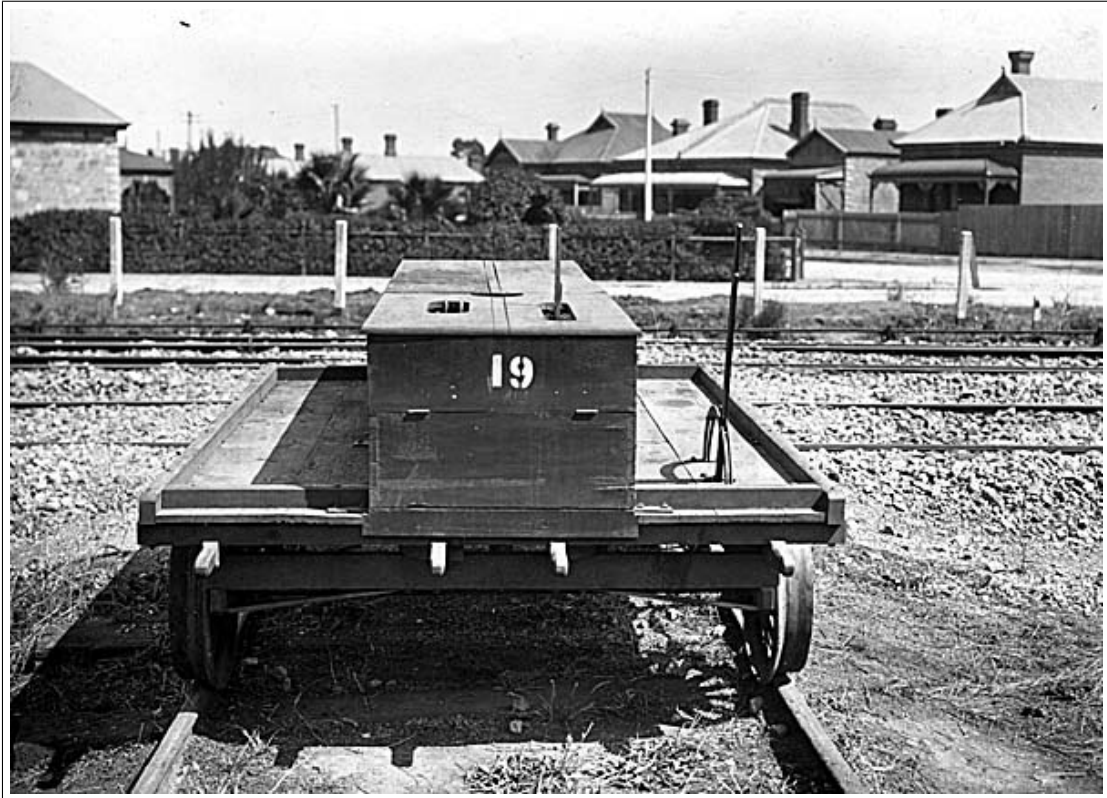
South Australian Railways - Ganger's Trolley similar to some the museum own - This unit was described by the railways as a motor section car (end view) - fitted with a 3 1 / 2 h.p. hopper water cooled two stroke engine. High tension (reversible) magneto ignition enabling car to be run in either direction. Belt drive with tension rack and lever. Speed 15 miles per hour ( NRM Collection )
