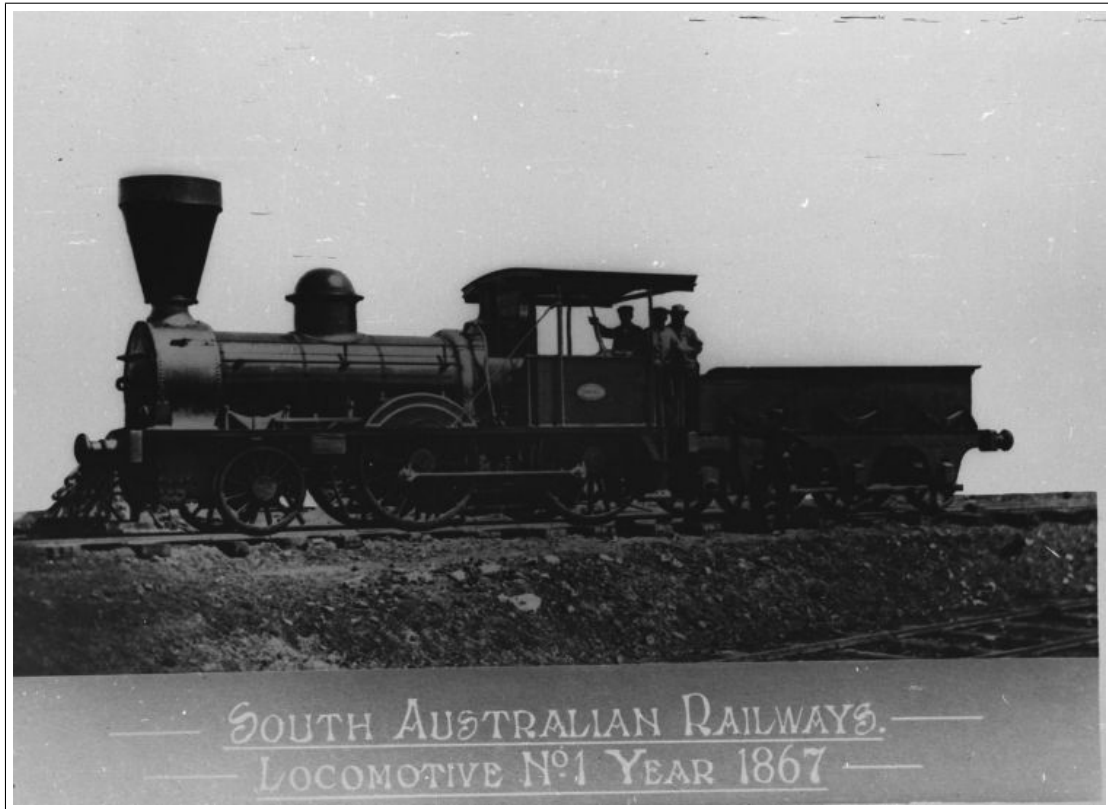
South Australian Railways - 2-4-0 Tank Locomotive Adelaide - Loco No. 1 after conversion from tank to tender loco - circa 1869 ( NRM Collection )
