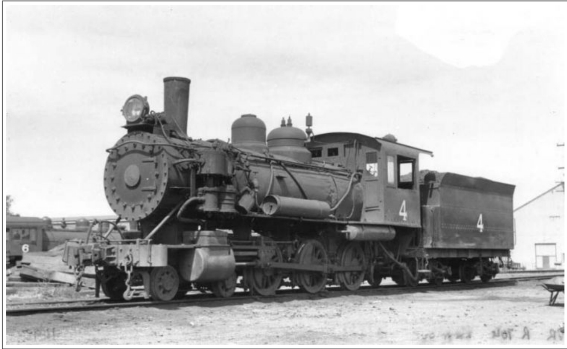
Broken Hill Proprietary Co. - Whyalla & Iron Knob Tramway - 4-6-0 Steam Locomotive No. 4 ( NRM Collection )
