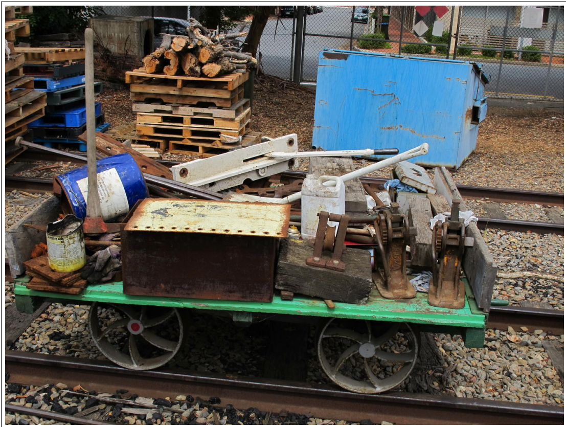
Unpowered gang trolley loaded with some of the gangs tools and track jacks - 12 February 2011 ( Chris Drymalik )
