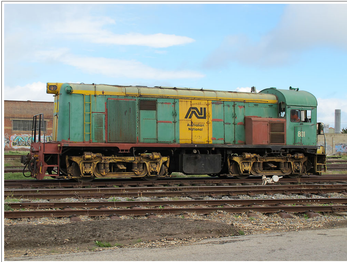
South Australian Railways 800-class Bo-Bo Diesel Electric Locomotive No. 801 at the museum - 29th May 2010 ( Chris Drymalik )
