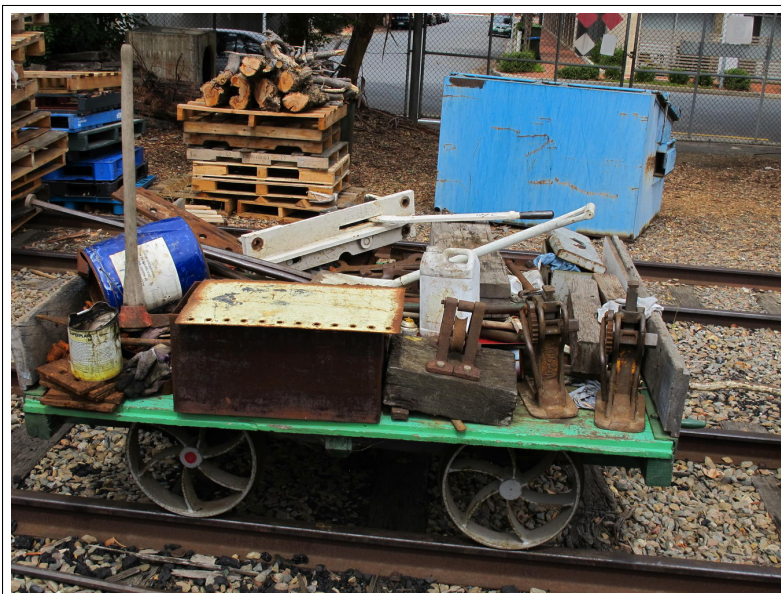
Unpowered gang trolley loaded with some of the gangs tools and track jacks - 12 February 2011 ( Chris Drymalik )
