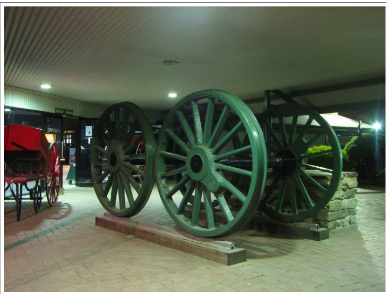
Locomotive wheels originally used on 2-4-0 Tank Locomotive 'Adelaide', 'Victoria' or 'Albert' ( A. Peters )
