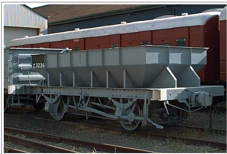
South Australian Railways - Z Class 4-wheel Steel Hopper Wagon No. 3236 ( NRM Collection )
